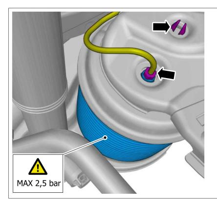
Reinstall the air line to the rear spring gaiter.
