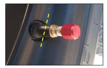
4. Using the tire machine, break the tire bead from the wheel bead seat. Allow sufficient space for the tire bead to clear the TPMS sensor.
