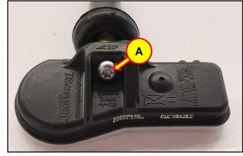
6. Install the new valve stem on to the sensor.
