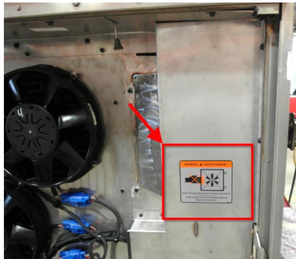
147. Install a second warning decal #069205 as shown on the radiator door.
