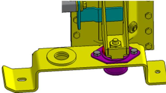
FIGURE 21: MOUNTING SUPPORT AFTER 180° ROTATION
