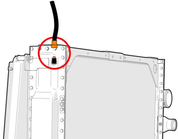
12. Cut the cable tie and disconnect **electrical connector** from the fan clutch. The remaining connector on the chassis cable will be capped and left in place.
