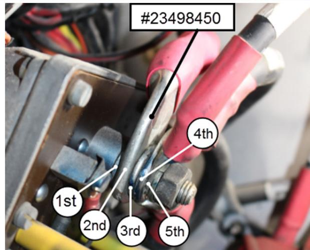
FIGURE 151: ON THIS PICTURE, CABLE #23498450 LUG IS IN SECOND (2<sup>ND</sup>) POSITION BECAUSE IT WAS LIKELY TO RUB ON THE HEAD OF ONE OF THE FOUR SCREWS.
