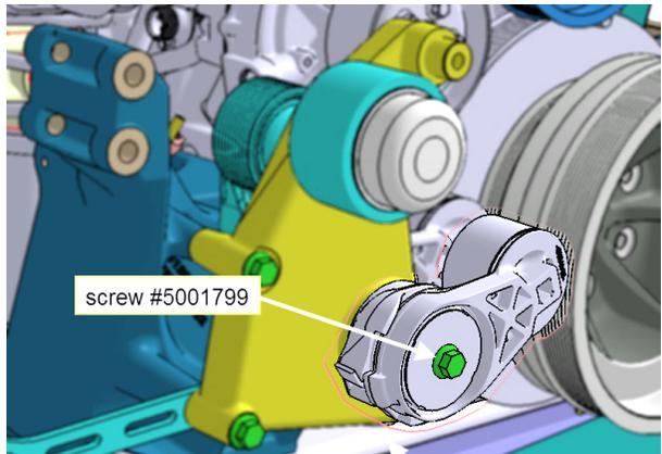
FIGURE 46: TENSIONER MOUNTING SCREW TORQUE : 48 lb-ft
