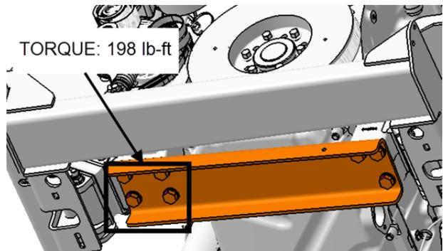
**FIGURE 35: FOUR (4) SCREWS UNDER THE REINFORCEMENT CHANNEL**
