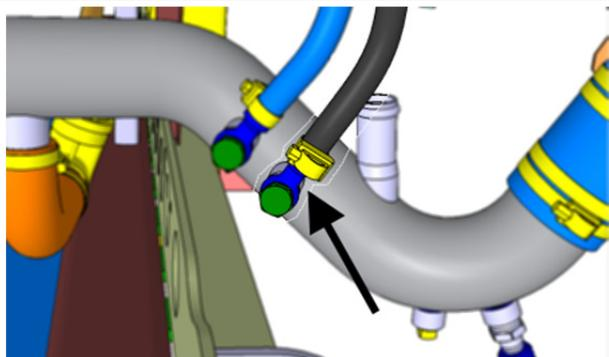
FIGURE 71: DEF INJECTOR COOLANT LINE RETURN HOSE
