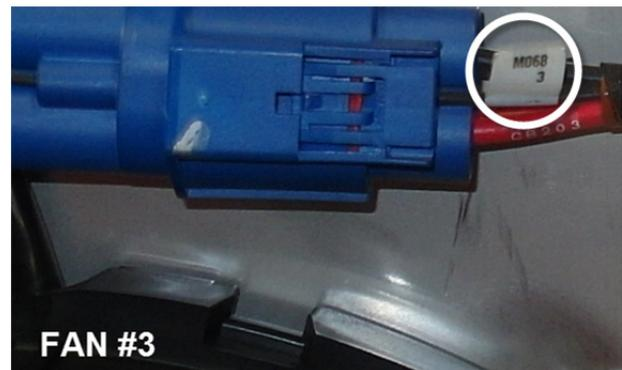
104. Snap the fan blue connector in the holes punched on the panel for that matter.
