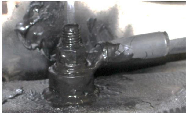
FIGURE 80: GROUND STUD WITH RUBBER COATING
