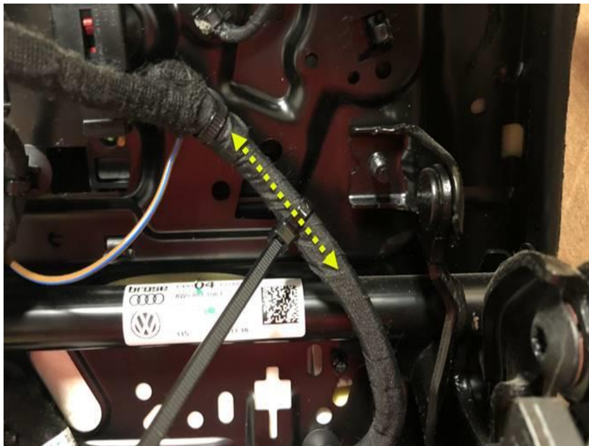
Figure 2. Attach the first cable tie in the yellow area.
