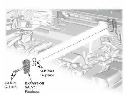
4. Connect the A/C lines to the expansion valve, and torque the bolt to **9.8 N·m (7.2 lb-ft)**. Make sure to replace all of the O-rings with new ones.
