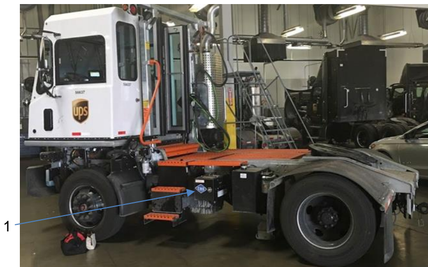
Figure 1. Fuel Management Module (FMM) (1) location on Tico CNG chassis.
