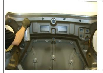
11. Once the plugs are removed, apply the cavity wax **remover** liberally to all of the cavities starting from the top down. Use ½ of the bottle, the other ½ is to be used for the second application.
