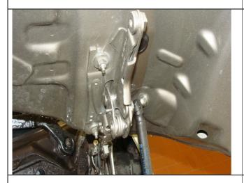
6. With hood safely supported, loosen nut (1) on both sides, but do not completely remove. Remove nut (2) completely on both sides.
