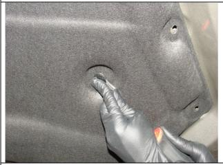
2. Raise hood and remove clips holding under-hood insulation using appropriate clip removal tool.
