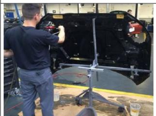
8. Remove hood completely from the vehicle and place into body panel hanger, or:
