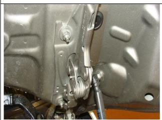
17. Re-install hood, all (4) tighten hood attachment (M8) nuts to 19 Nm.
