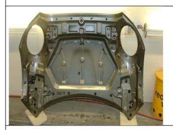
9. If body panel hanger is not available, the hood can be rested in the position shown. Use foam blocks as shown to prevent damage to the corners and surface of the hood.
