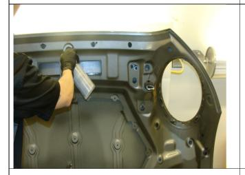
14. Using the remaining ½ of the bottle of cavity wax **remover**, apply again from the top down. Repeat steps 11 through 13.
