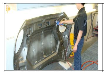
13. Using compressed air, dry the hood from the top down.
