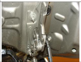
5. Install appropriate tool to support hood and disconnect hood strut at upper mount on both sides.
