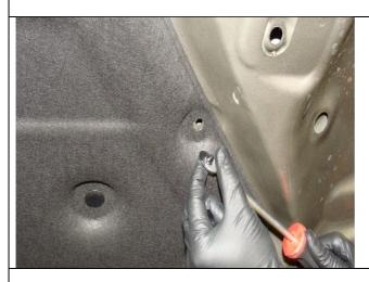
3. Remove clips for under-hood insulation and remove insulation completely.
