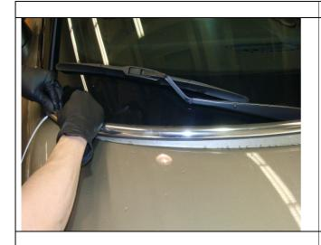
Remove chrome trim from rear of hood to prevent damage. Refer to "51 13 085 Removing and installing/replacing trim strip on engine compartment lid (cowl panel).
