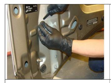
10. Using suitable plastic tool, remove all rubber grommets and body plugs on the underside of the hood (12 total).
