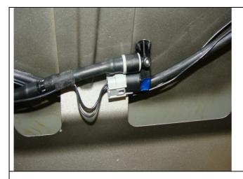
4. Disconnect and remove washer hose and both washer nozzles.
