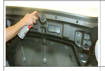
15. Once the hood has been thoroughly rinsed and dried, re-apply cavity wax to cavities in the hood. Start from the top and work down spraying a small amount into all holes and cavities.
