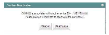
**Action to take**: Verify the Chassis and ESN or IMEI and attempt the submittal again. If the existing IMEI in the vehicle and the VIN are correct, and the IMEI is to be replaced, select "**Deactivate**." This will deactivate the existing IMEI in the vehicle.
