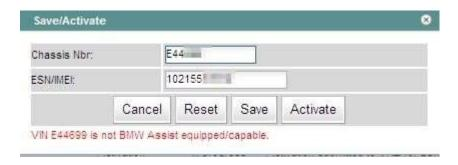
Action to take: Verify the Chassis, and the ESN or IMEI on the telematics control unit's label and attempt the submittal again. If error persists, check for presence of SA 639 or 6NL or 6AE on the vehicle order or for history of a retrofit. If not present, the vehicle is not equipped.
