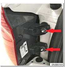
2. Visually inspect the mounting area of the tail light as shown to the left.
