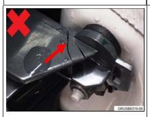
Reference the photos to the left showing examples of cracks that are NOT acceptable and which require tail light replacement or repair.
