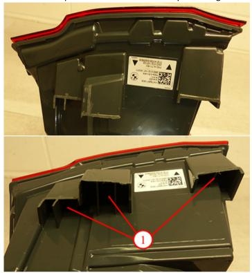
5. De-burr all of the plastic edges from cutting during the previous steps. Using compressed air, ensure that all of the plastic debris is removed. The tail light must be completely free of any cutting remains.
