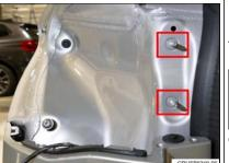
8. With the damaged rear light removed from the vehicle, the tail light mounting studs and vehicle body **MUST** be cleaned to remove residual manufacturing oil.
