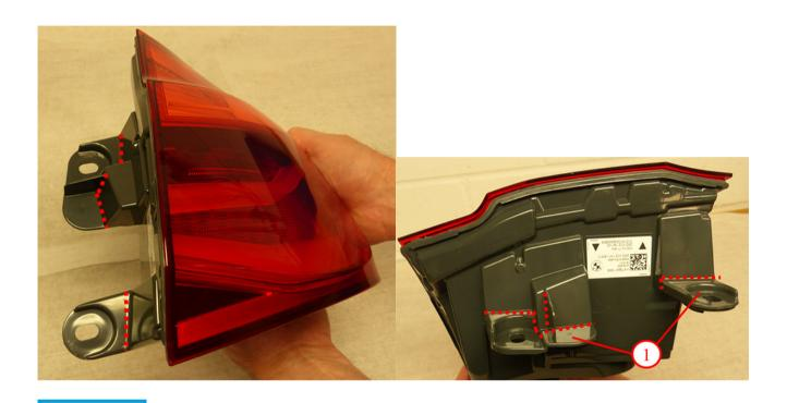
Note: The aid of a second person may be needed to hold the taillight while cutting.
