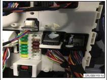
2. Perform visual inspection of BDC and connectors looking for cavity wax.
