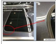
Excess butyl sealant has leaked out from underneath the seal of the rear stationary sunroof glass.
