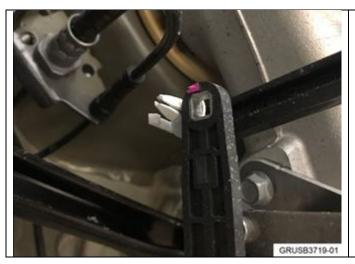
The ride height sensor linkage became disconnected.
