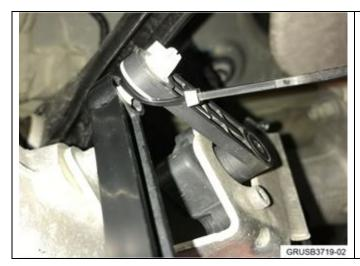
Reconnect the ride height sensor linkage, and secure with a wire tie through the center hole of the sensor arm.
