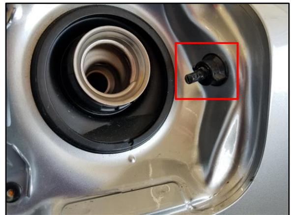
9. Remove the fuel door lock switch retainer by rotating it clockwise ¼ turn and pulling the retainer toward the front of the vehicle.
