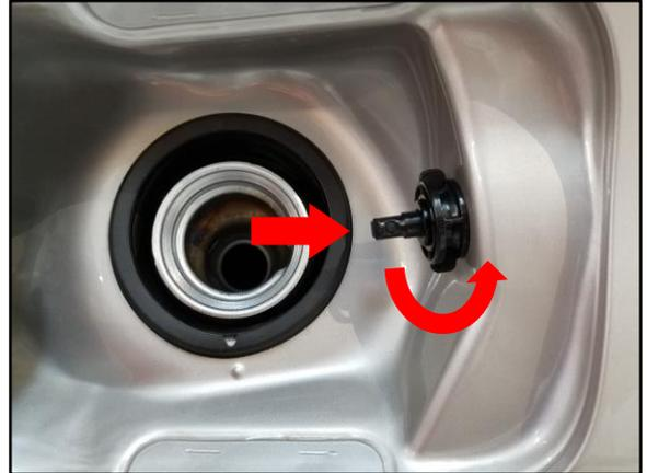
11. Install the fuel door lock switch cover.
