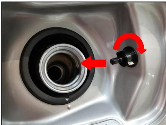
Figure 8. Retainer Removed
