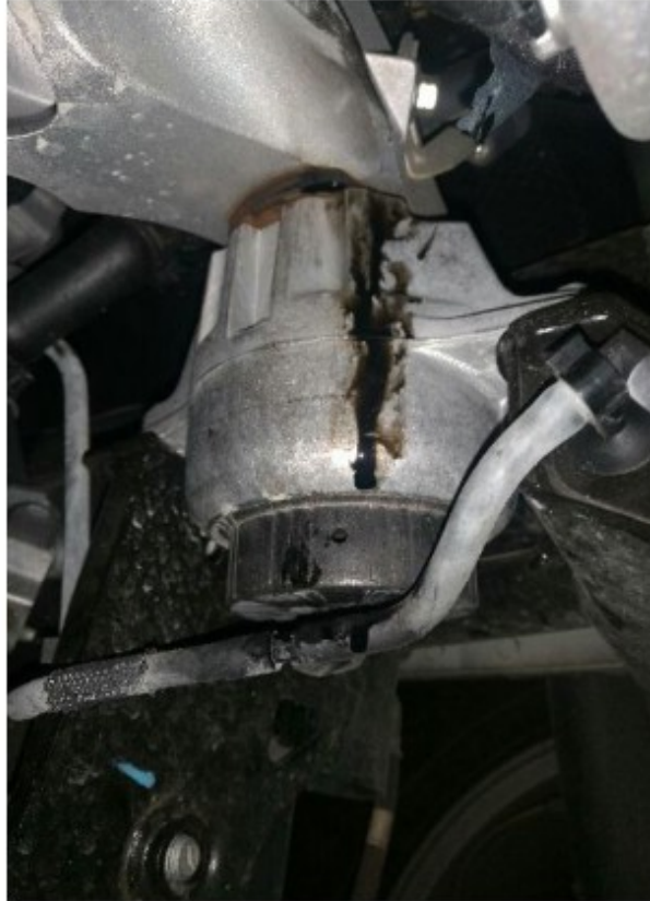
Excessively worn and/or leaking active engine mount.
