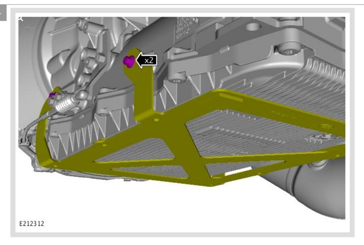
Remove the 2 transmission heatshield mounting bracket retaining bolt(s).
