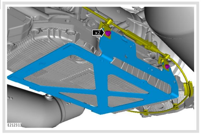
Remove the transmission heatshield mounting bracket retaining bolt(s).
