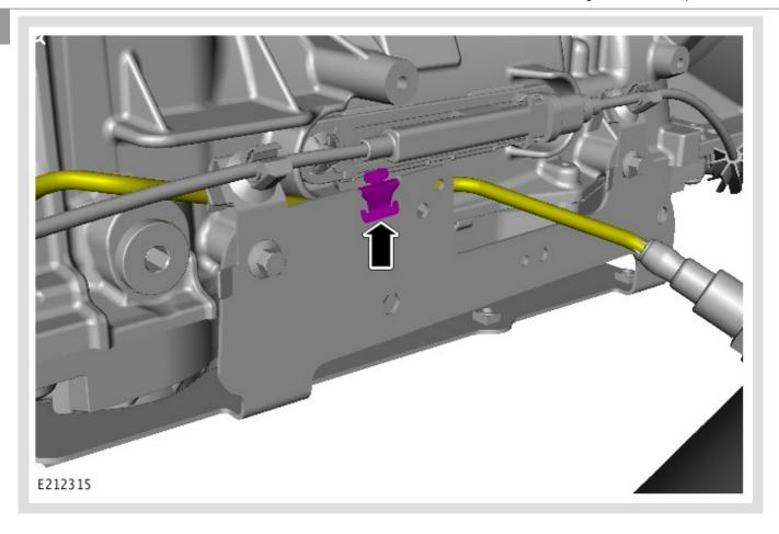
Release the Heated Oxygen Sensor (HO2S) electrical wiring harness from the retaining clip(s).
