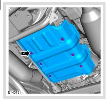
Remove the transmission heatshield retaining bolt(s).
