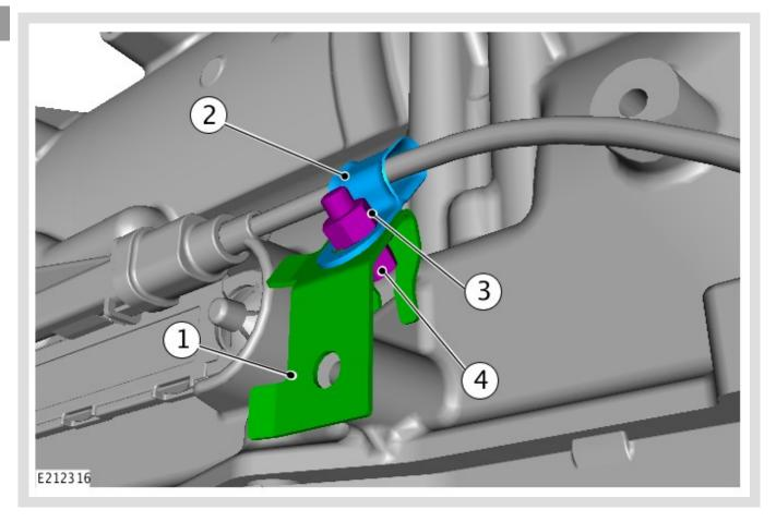
Install the EPB cable mounting bracket as shown:
