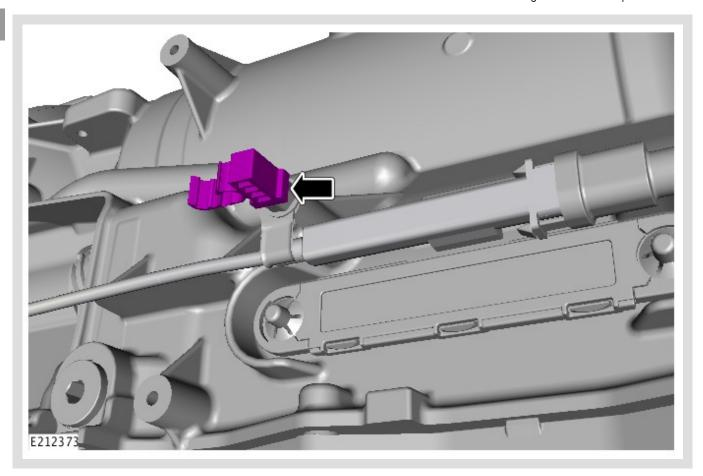
Install the HO2S electrical wiring harness retaining clip(s).
