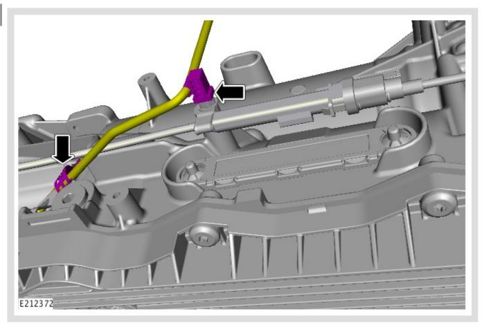
Install the HO2S electrical wiring harness.
