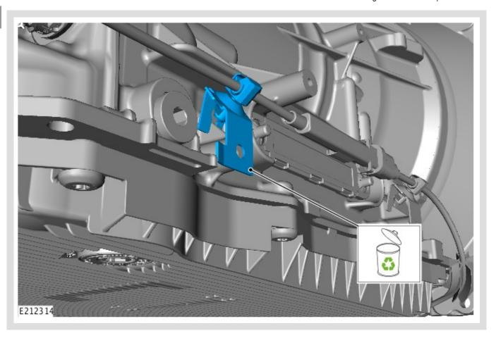
Remove and discard the <u>EPB</u> cable rear mounting bracket.
