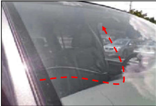
Single crack with no impact mark: Warranty
