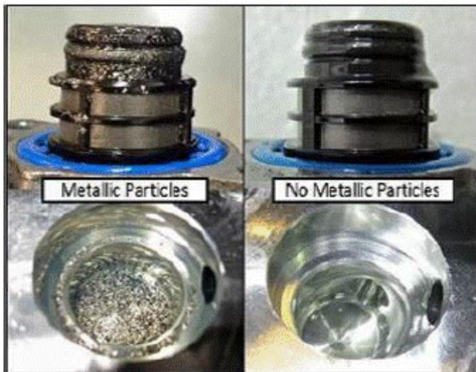
Figure 3. N290 Fuel Metering Valve and Valve Bore
