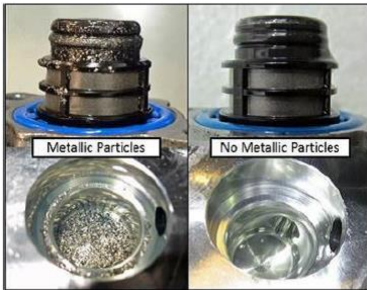
Figure 3. N290 Fuel Metering Valve and Valve Bore
