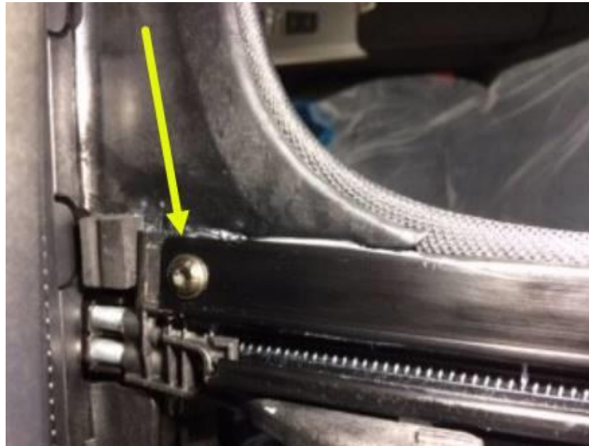
Figure 8. Loosen the bolt and apply lube paste between these panels and under the bolt head. Reinstall the bolt and torque to 5Nm.
