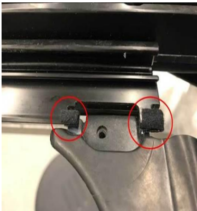
Figure 7. Apply felt tape on points shown.
