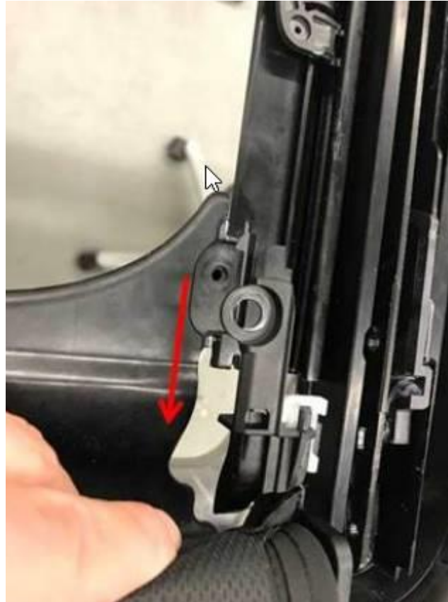
Figure 4. Slide roller shade backward.
