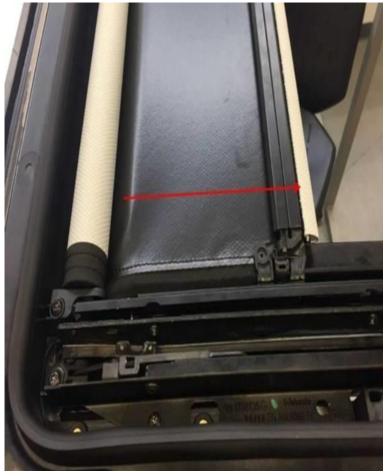
Figure 1. Closing the roller shade.
