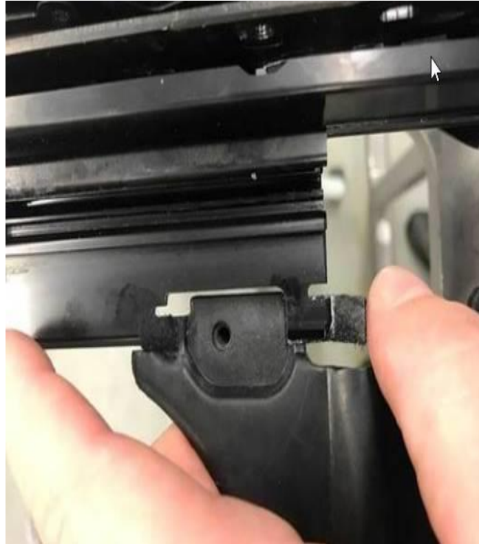
Figure 6. Applying felt tape.
