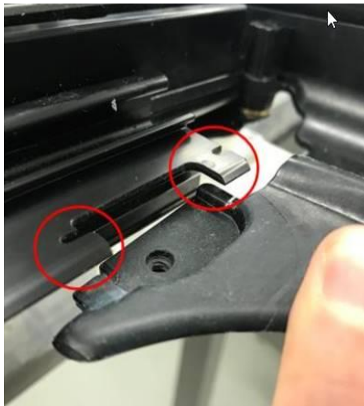
Figure 5. Removing the roller shade.
