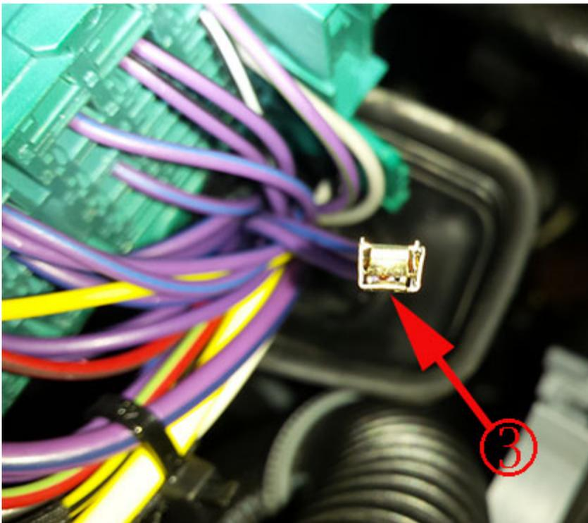
**Notice Tighter tension of terminal after repair**
