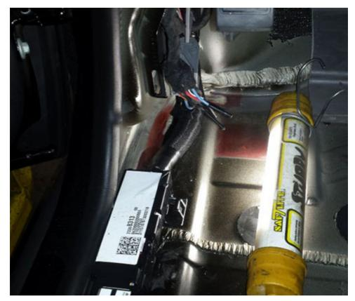
The other area is under dash in the left and right side vertical seams. Reseal as needed
