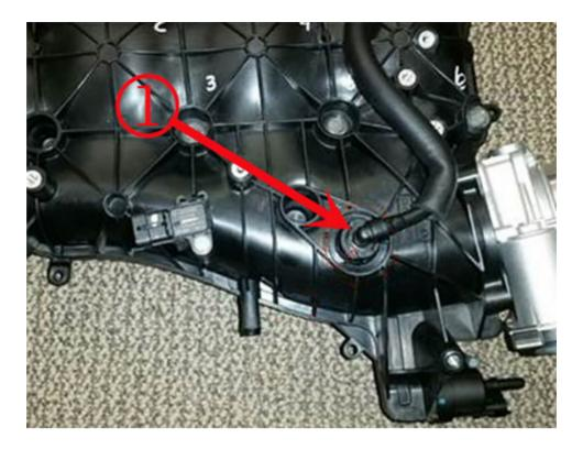
Detach foul air tube from connection shown above at arrow 1 and plug both sides
