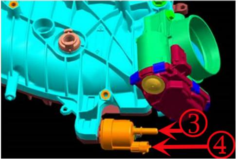
4. Restart the vehicle then place your finger or a vacuum gauge over the open port on the purge valve.
