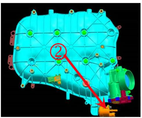
3. Disconnect vacuum hose and power supply from purge valve (see below)
