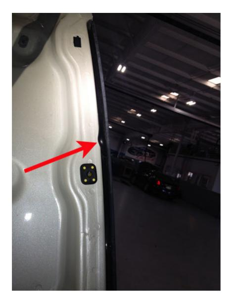
2. Install a 5mm X 5mm ( $3/16 \times 3/16$ ) piece of closed cell foam tape along the entire length of the tail light assembly, as shown below.
