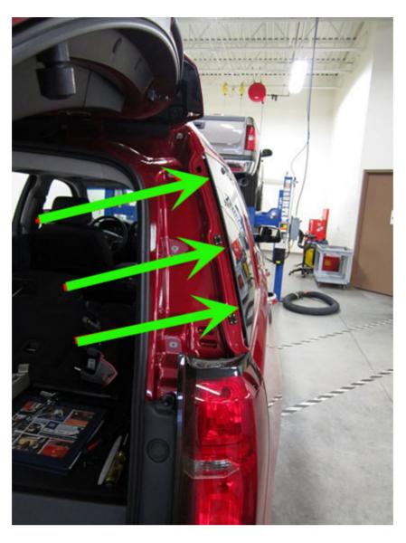
2. The gap between the rear tail light assembly and the quarter panel, as shown below.
