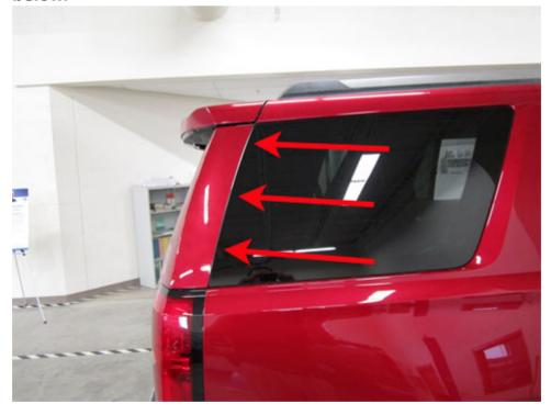
Excessive urethane from the quarter glass installation may not allow the exterior "D" pillar trim to fit properly against the rear quarter glass, as shown below.
