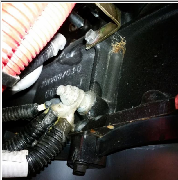
Figure #3: Ground Stud on engine block (A26)
