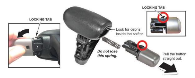
6. Insert the spring into the shift knob button, and slide in the new shift knob button until it clicks into place.
