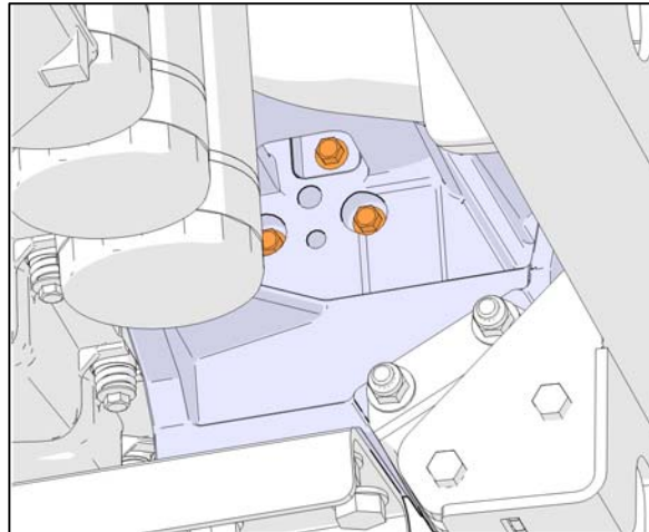
FIGURE 49: IDLER / TENSIONER ASSEMBLY MOUNTING SCREWS
