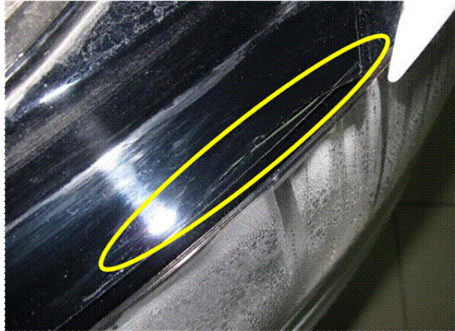
Figure 5. Upper headlight housing is cracking.
