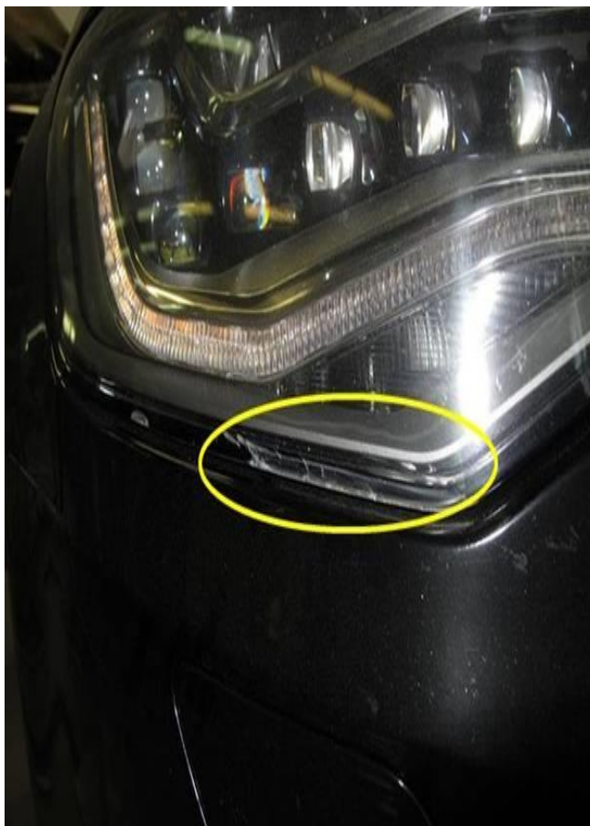
Figure 3. Lower headlight lens is cracking.
