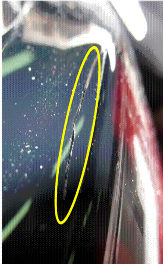
Figure 4. Upper headlight housing is cracking.
