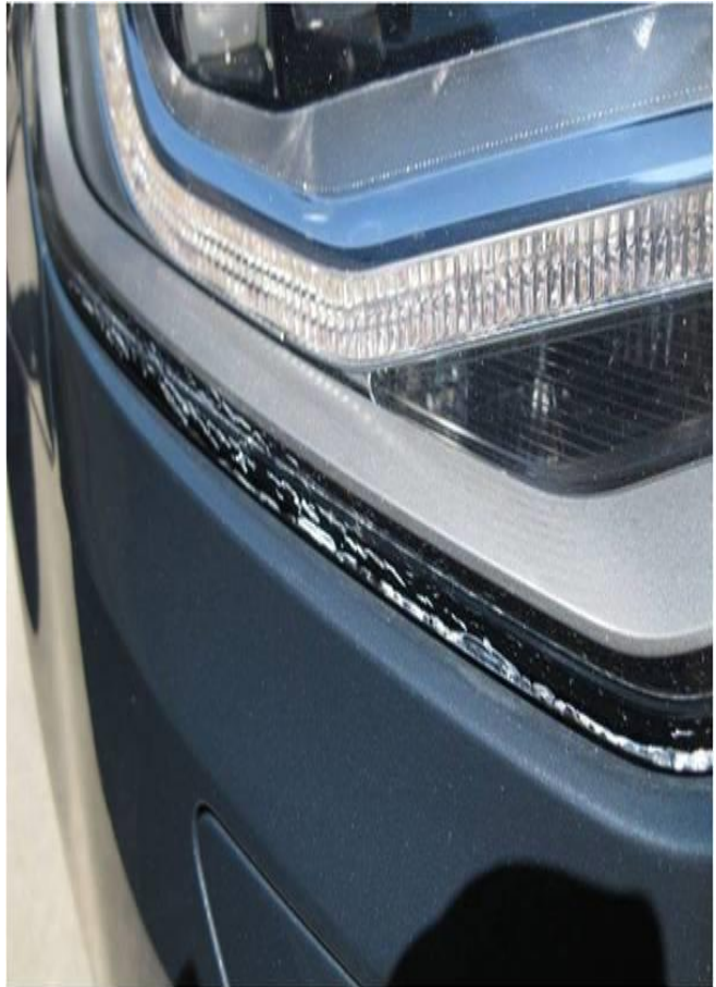
Figure 2. Lower headlight lens is cracking.
