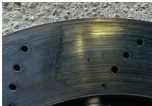
Figure 2. Deposits on the brake disc.
