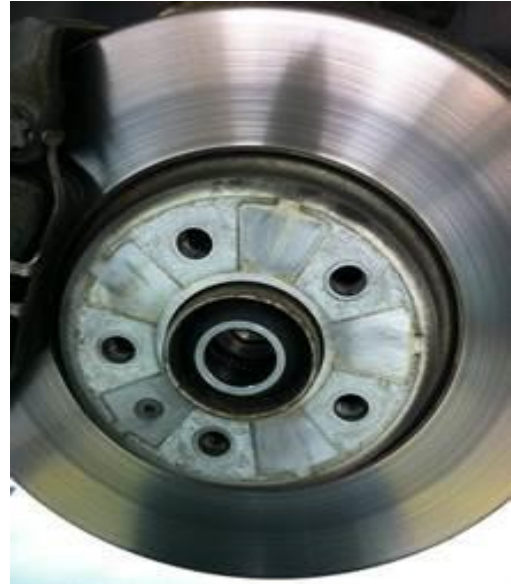
Figure 3. Brake disc with heat marks.
