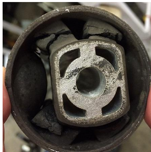
Figure 8. Damaged suspension bushing.
