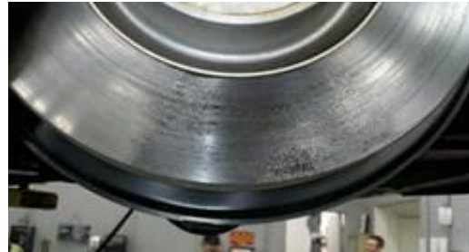
Figure 5. Pad marks on the brake disc.
