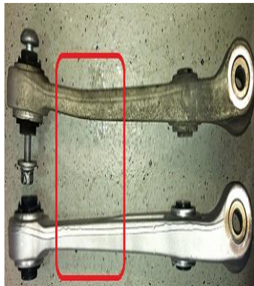
Figure 9. Damaged suspension link.
