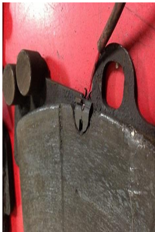
Figure 7. Worn brake pad.
