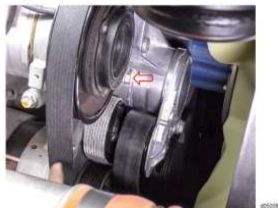
Figure 2: Accessory Drive Arm Pinned (M10x50 mm bolt)
