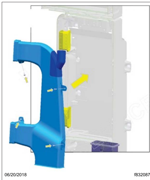
Fig. 9, Installing the Cabinet Ducting
