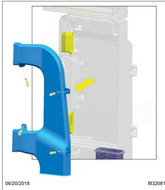
Fig. 2, HVAC Cabinet Ducting
