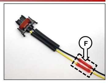
Crimp the butt splice connectors at two (2) locations (G) of each connector for both wires.
