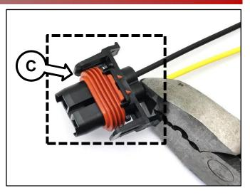
6. With a pair of wire strippers, strip 10mm (0.4") from the two (2) low beam bulb wiring harness.
