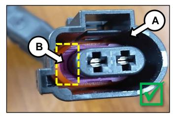
If retainer (B) is unlocked as shown, then slide the lock retainer towards the center of the connector as shown using small flathead screwdriver.
