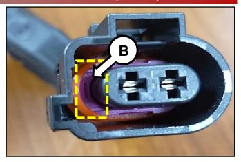
Re-install the EPB connector (A) at the caliper (verify clicking sound from locking tab) and perform push/pull to confirm the connector is secured.
