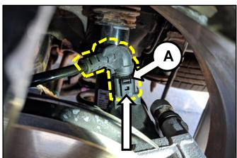
3. Check the terminal retainer (B) located inside of the connector (A).
