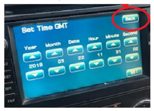
In order to get out of the diagnostic mode the vehicle will need to be turned off and RAP cancelled for a minimum of 5 min. After the 5 minutes has passed the dealer should be able to turn the vehicle on and the clock should display.
