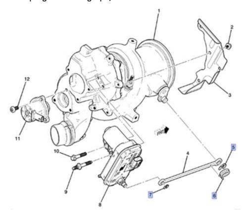
If you find a missing wastegate lever retaining clip either at the actuator or wastegate valve. These retaining clips and anti-rattle spring may be available through CCA Parts, if so, then install the missing retaining clip and anti-rattle spring if needed and evaluate.
