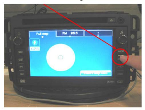
4. At the top of the display, press the "display" soft key
