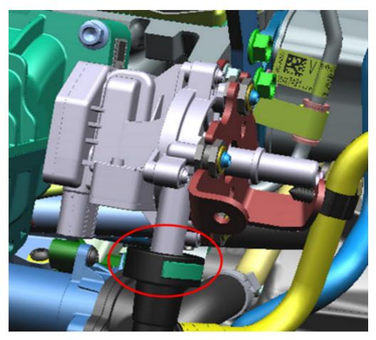
11. Look for a leak at pump to tube connector (o-ring):
