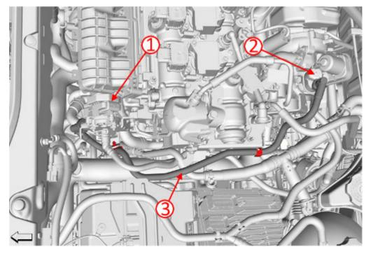
4. Separate the purge tube (3) at the purge valve (2).
