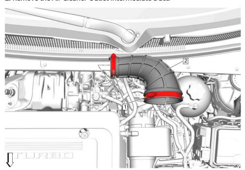
3. Remove the Turbocharger Outlet Duct Connector.
