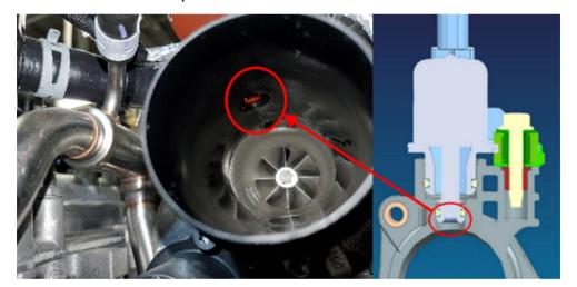
14. Look for an internal valve leak past the valve O-ring into the adaptor, DO NOT REMOVE valve from adaptor:
