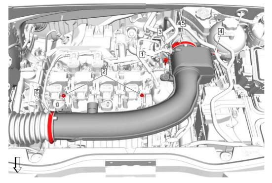
2. Remove the Air Cleaner Outlet Intermediate Duct.
