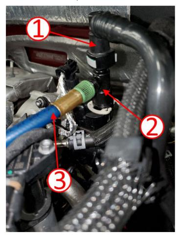
12. Look for leak at the purge tube (1) to T-fitting (2):
