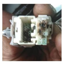
If there is corrosion, clean the connector using a commercially available electrical cleaner and inspect the area for source of a water leak.
