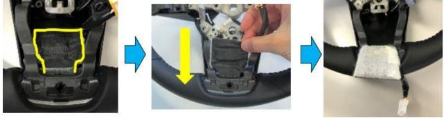
9. Apply the aluminum tape to the lower right corner of the backside of the steering wheel heating element, as shown below.
