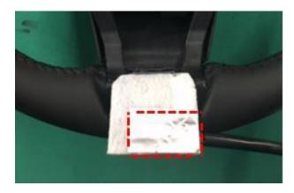
10. Apply double-sided adhesive tape to the backside of the steering wheel heating element, as shown below.
