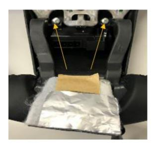
12. Reinstall the steering wheel heating element to the core cover.
