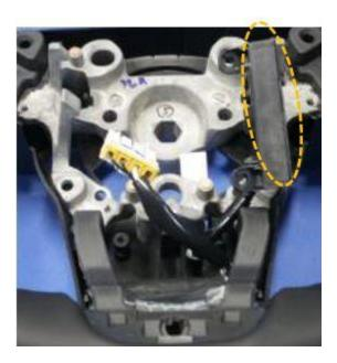
8. Peel off the steering wheel heating element from the core cover, as shown below.
