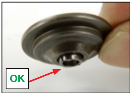
Both keepers are protruding the same amount from the bottom of the retainer.
