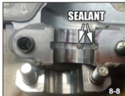
Sealant Plugging Lubrication Channel
