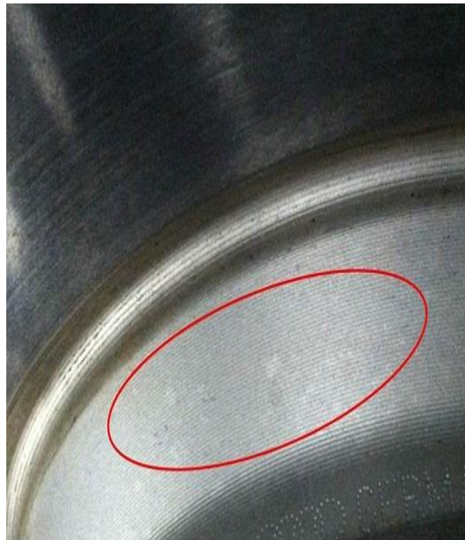
Figure 4. Small spots and discoloration due to chemical contamination from the cleaner that was sprayed directly onto the disc.
