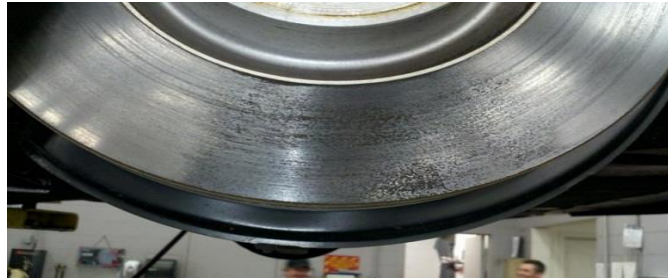
Figure 5. Brake pad material has transferred to the discs.
