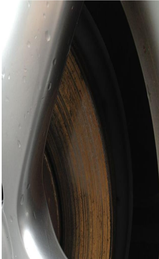
Figure 1. Disc covered with rust.
