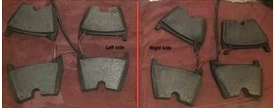
Figure 11. Example of pads without adhesive (mark position for reinstallation if not replaced).
