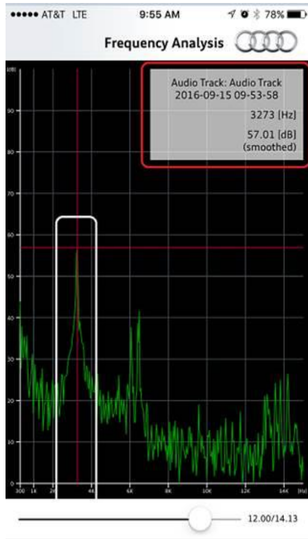
Figure 10. Typical brake squeal frequency recording.
