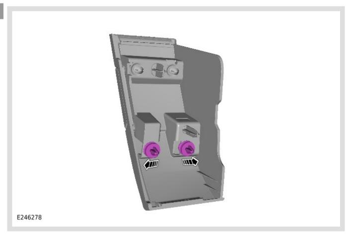
Install retaining clip(s), LR035841, into the lower.
