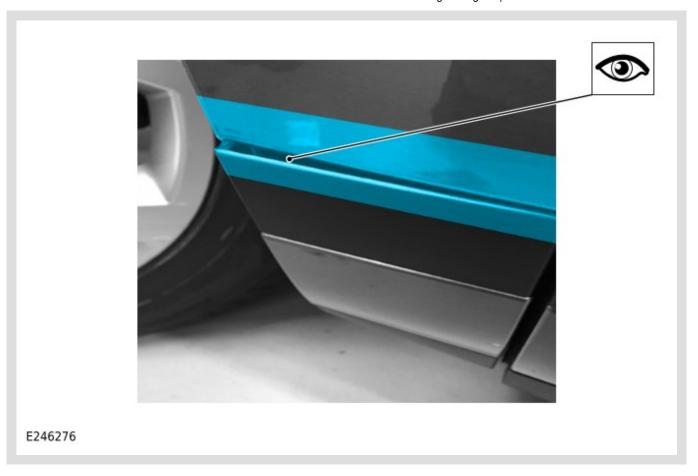
Inspect the alignment between the front fender lower cladding and the bottom of the fender.
