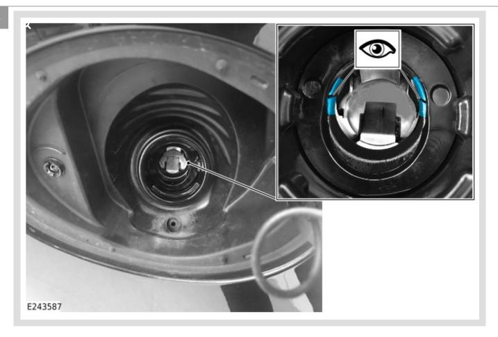
Inspect the fuel filler neck for signs of cracking as shown.
