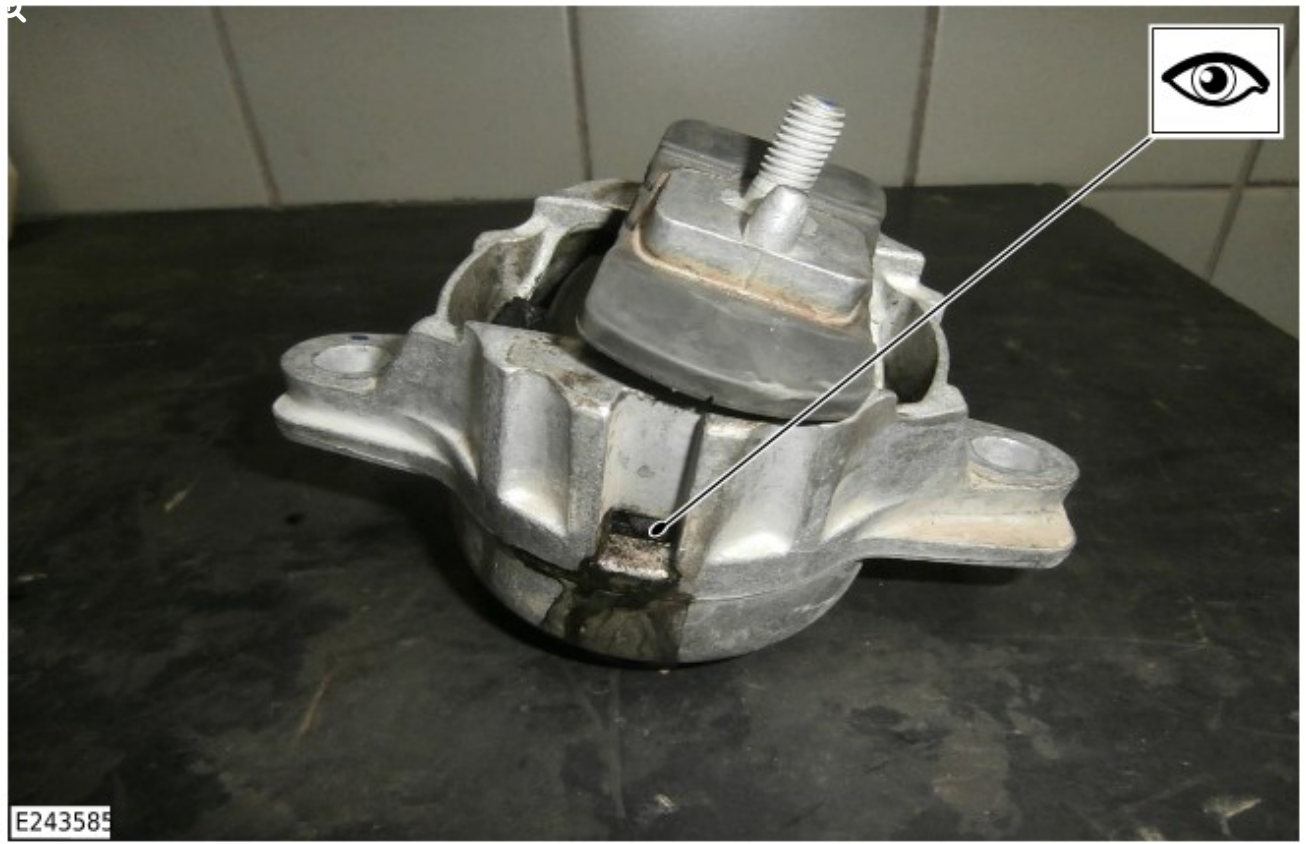
Excessively worn and/or leaking active engine mount.
