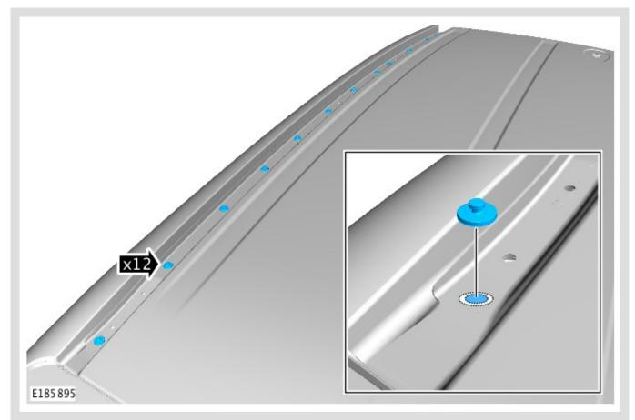
Install the new roof molding studs in the positions previously applied with bonding glue.
