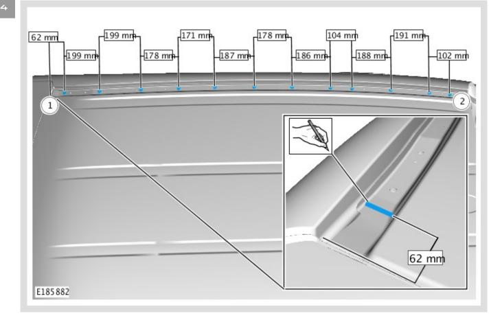
Starting at the windshield (1) and moving towards the rear of the roof panel (2), use a suitable marker to mark the roof channel in the positions indicated.
