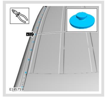
Use a suitable tool to remove the 12 roof molding studs.
