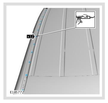
Apply the bonding adhesive to the areas previously marked in Step 5.
