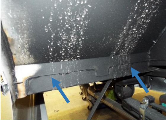
As built; No Sealant in Wheelwell Mud Flap Removed
