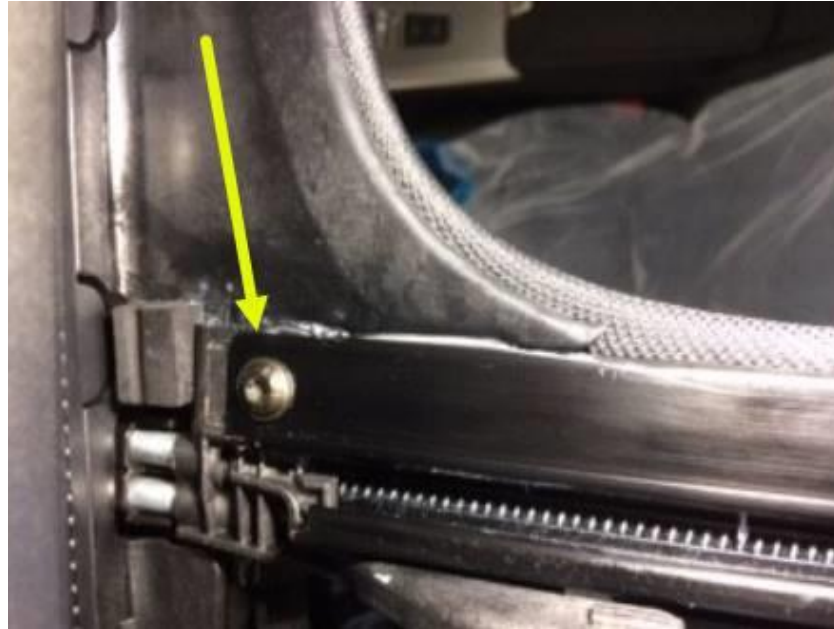
Figure 8. Loosen bolt and apply lube paste between these panels and under the bolt head. Reinstall the bolt and torque to 5Nm.
