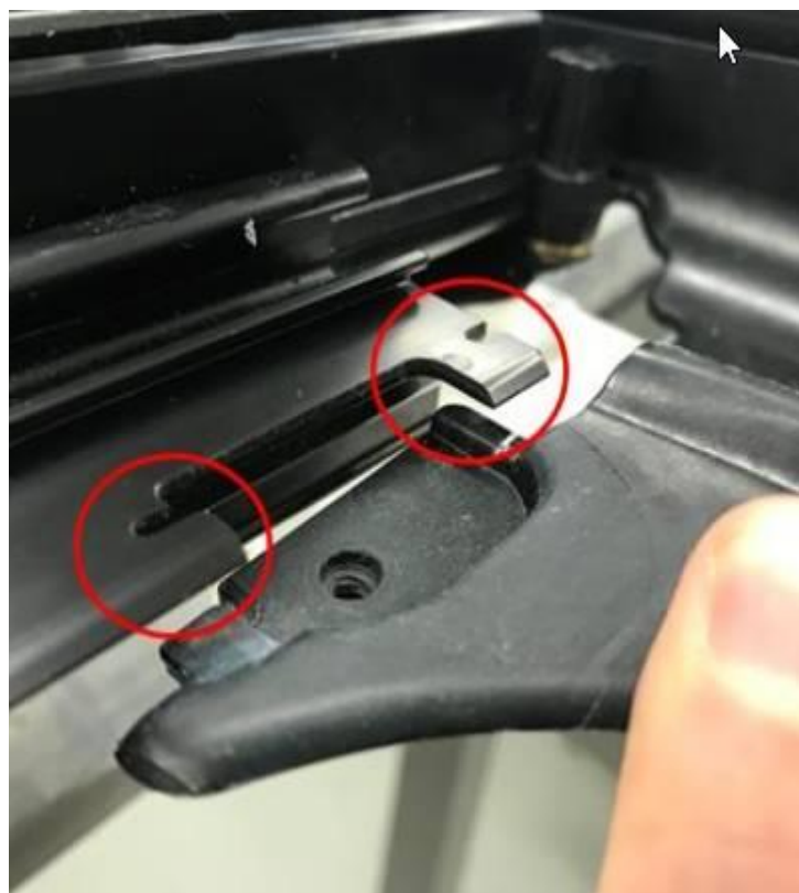
Figure 5. Removing the roller shade.
