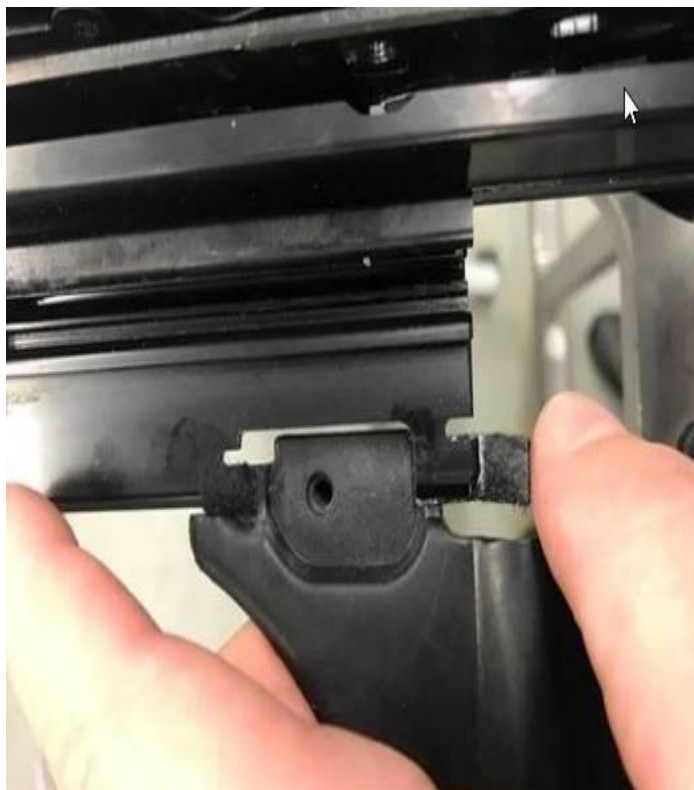
Figure 6. Applying felt tape.
