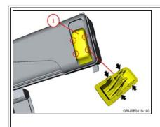
2. Install 2 new release buttons by pressing the button's locking tabs into the roller cover.
