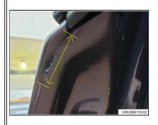
3. Wipe off excess cavity preservation spray, so that only a small coating is left on the door seam as shown below:
