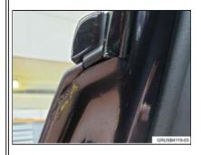
4. Open and close the door multiple times. Remove any excess cavity protection spray that may transfer onto the rear door rubber seal as the door is closed.
