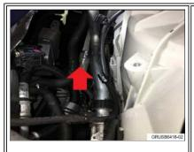
The steering shaft can contact the heater hose, possibly wearing through the hose.
